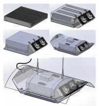
Specialized sheet metal locking mechanisms and extruded thread features were designed into the heatsink, which eliminated the need for excess machining and hardware. Aavid's experience with manufacturing processes meant we could add design details that reduced the cost of material, component manufacturing. and assembly.
